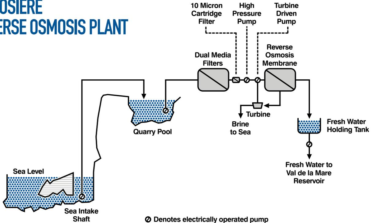
A deep sea water intake shaft and tunnel constructed below the mean low tide level on the foreshore allows sea water to be pumped at all states of the tide, which can vary by as much as 12m. A macerator device in the sea water intake shaft chops up seaweed and other large matter. The sea water is discharged and stored into the quarry pool, which allows settlement of any unwanted debris rather than it floating to the surface.
