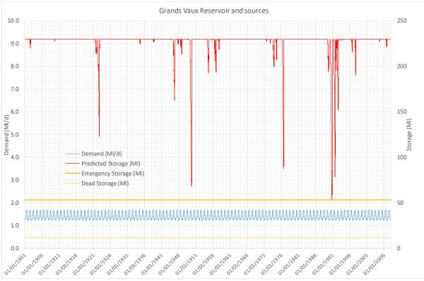
Figure C.7 Predicted raw water storage for the Water Works Valley system from 1901 to 2007 with demand at hydrological yield
