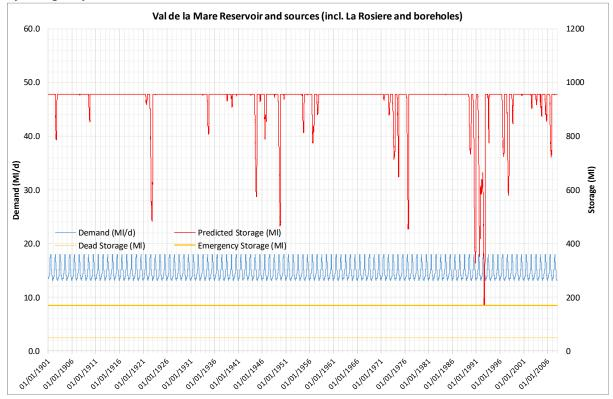
Figure C.9 Predicted Jersey Water total raw water storage from 1901 to 2007 with demand at hydrological yield
