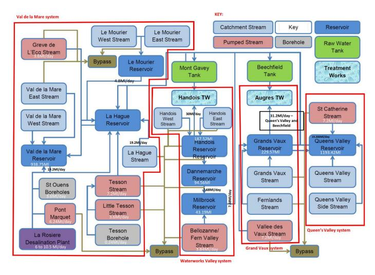
$<sup>^{\</sup>rm 1}$  N.B. The links between the raw water assets shown in the schematic are indicative only.
