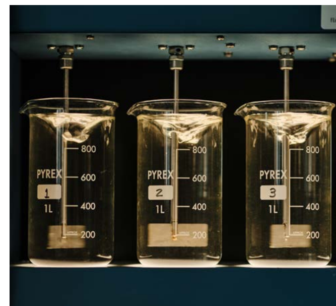
Treatment process optimisation by jar testing
