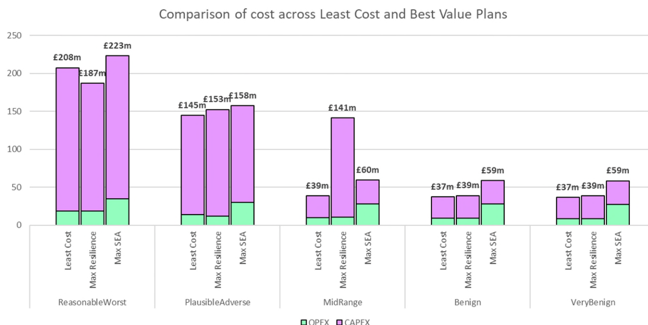
Figure 2-11 – Comparison of total NPC (£m) for the least cost strategy and the maximised Resilience and SEA runs. The Best-Value runs were constrained such that the total expected cost across all futures was not more than 20% greater than the total expected least cost strategy.
