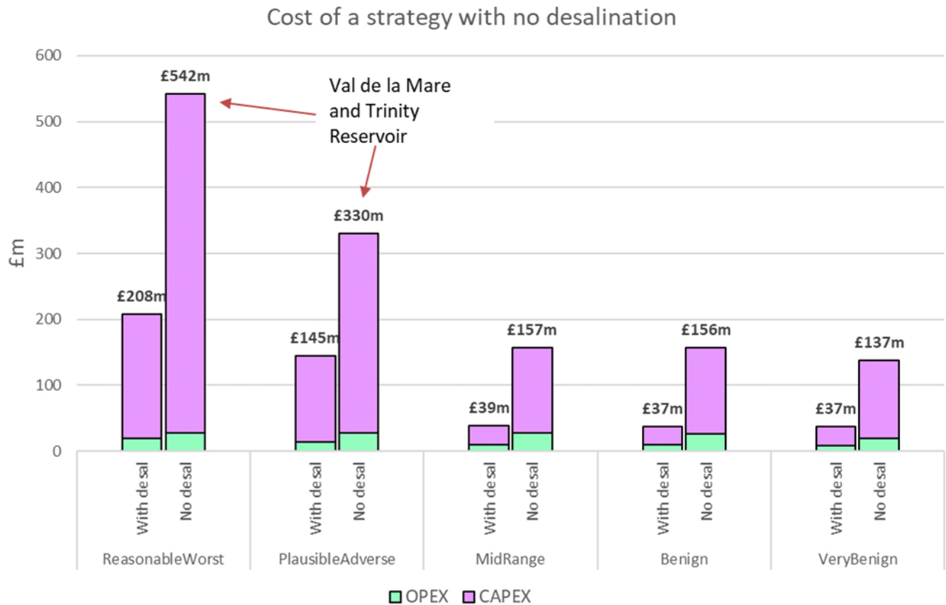
Figure 3-3 – Comparison of total NPC (£m) for the least cost strategy with La Rosiere desalination extension available and without the desalination extension option.
